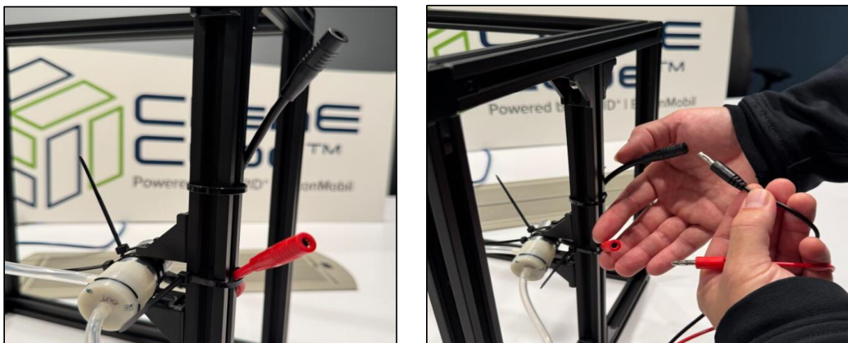
Figure 2: Connection Points for Power for Cube - Notice the example cube is providing female banana jack connections.
